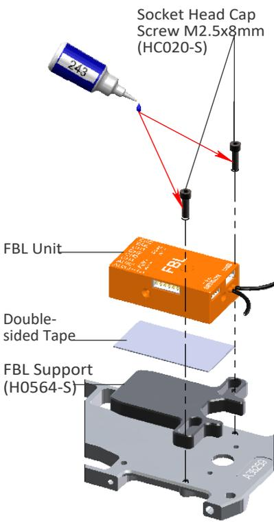
Fig. 2 shows the unit mounted on the support H0564.
