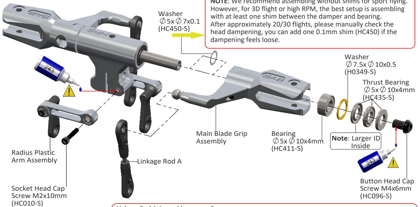
**NOTE:** We recommend assembling without shims for sport flying. However, for 3D flight or high RPM, the best setup is assembling with at least one shim between the damper and bearing. After approximately 20/30 flights, please manually check the head dampening, you can add one 0.1mm shim (HC450) if the dampening feels loose.
