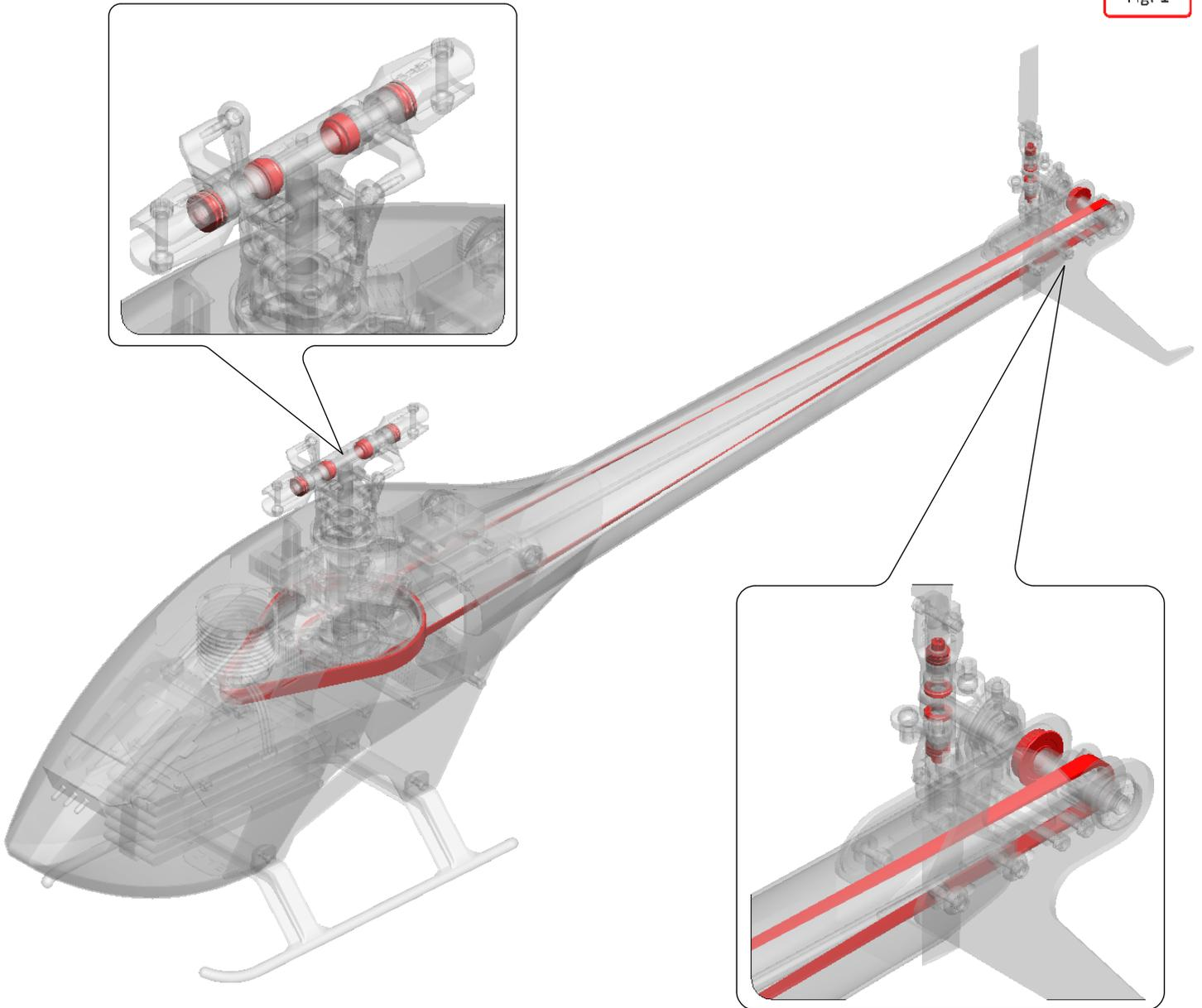
\*The lifespan of these components varies according to the type of flying. On average it is recommended to check these parts every **20** flights. In some instances, based on wear, these parts should be replaced every **100** flights.
