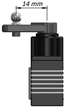
Uniball M2  $\varnothing$  5H6 (H0064-S)      Socket Head Cap M3x6mm (HC044-S)
