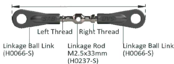
(Initial length for the rods from the swashplate to the blade grip.)
