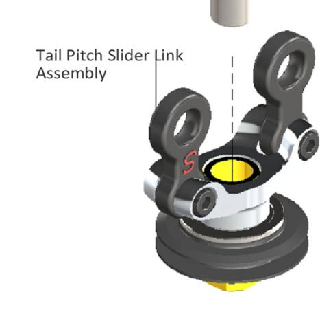
**Montage Schiebbehülse (Tail Pitch Slider)**
