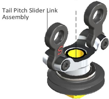
**Montage Schiebbehülse (Tail Pitch Slider)**
