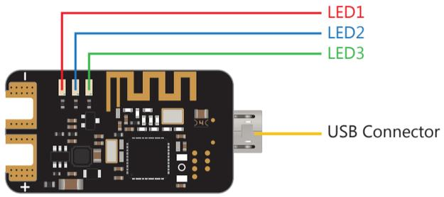
**Power:** Input voltage 2S~7S LiPo battery (6-30V)
