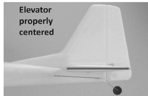
Then observe the elevator to ensure it is properly centered as shown below.
