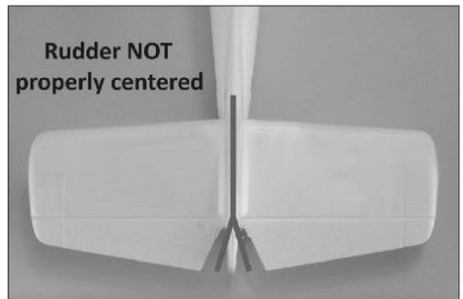
Observe the rudder to ensure it is properly centered as shown below.
