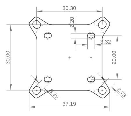
Maximum outside dimensions:  $37.2 \times 37.2 \text{ mm}$ , without outside tips  $30 \times 30 \text{ mm}$  Mounting hole arrangement:
