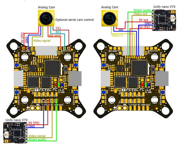
Note: RX and TX connection is only used for cameras which support serial connection
