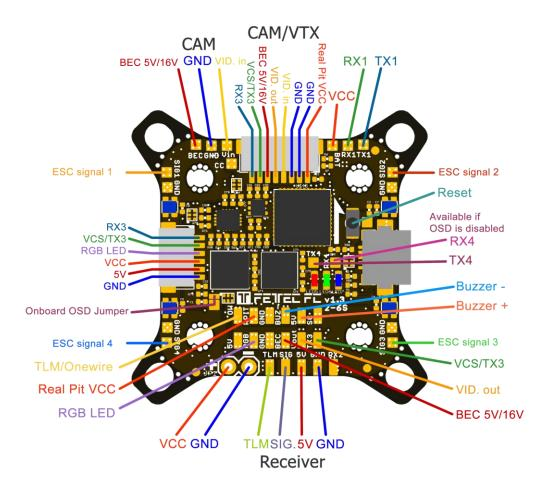
The 8 pin connector combines all necessary connections for analog or digital VTX and camera. It includes:
