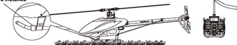
Rubber skid stoppers installed 裝上避震墊圈
