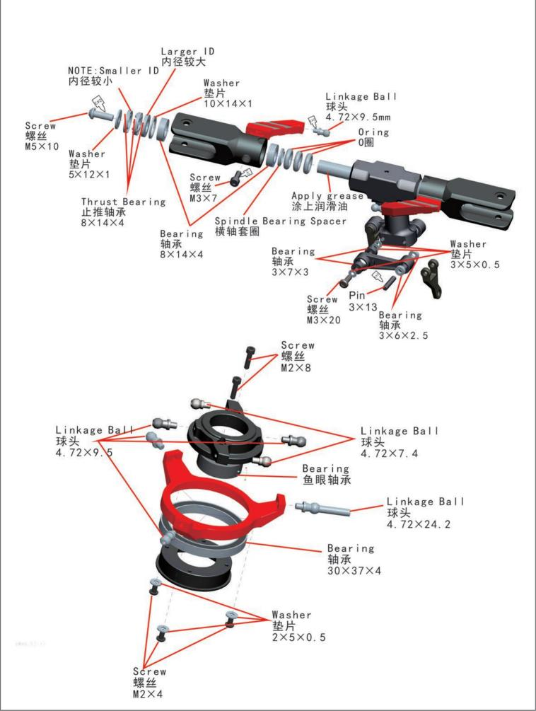
Apply a little amount of 243 243 **BB-1** thread lock when fixing a metal part 螺丝需上螺丝胶 Bearing 轴承 3×7×3 Note the direction 凸台朝向轴承 Pin\_ 3×17 (BB-1-1) (BB-1-2)Flat Head Cap Screw 平头螺丝 M2.5×6
